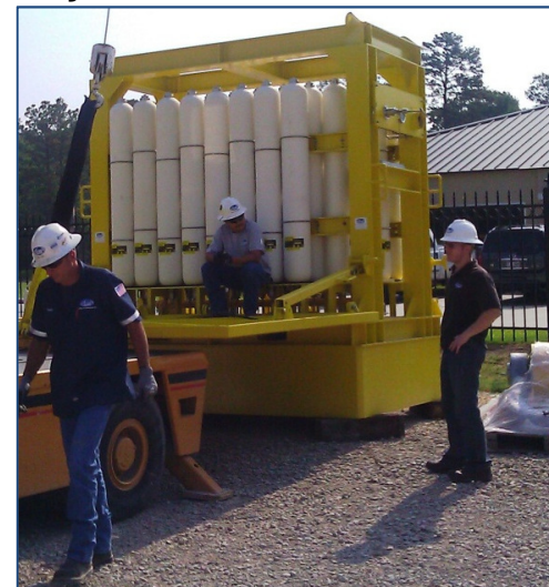
Hydraulic Accumulator Skid
