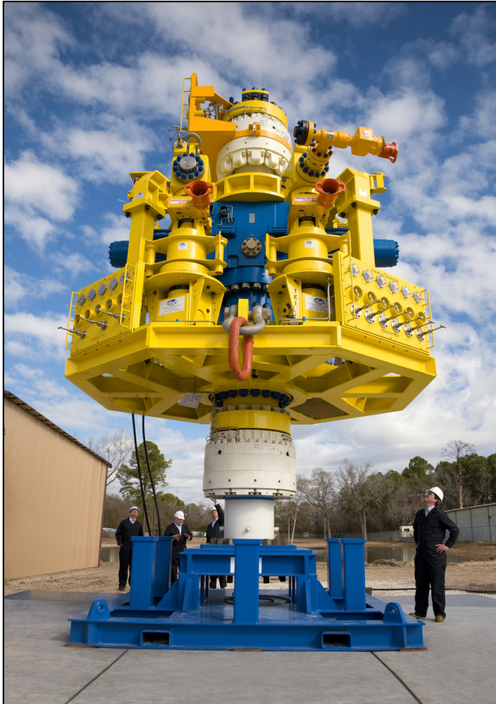
15 ksi Capping Stack
