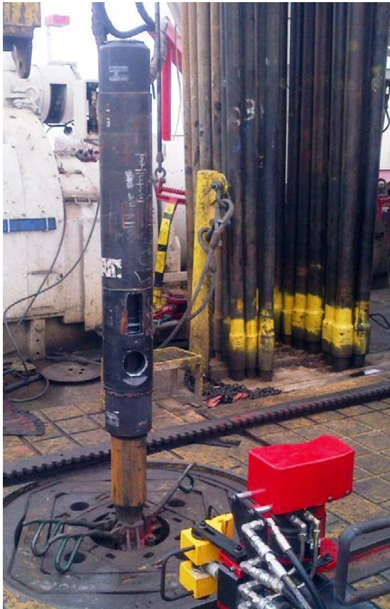
CFS sub – One sub per stand is needed. Subs are pre-assembled to stands before putting them in derrick.
