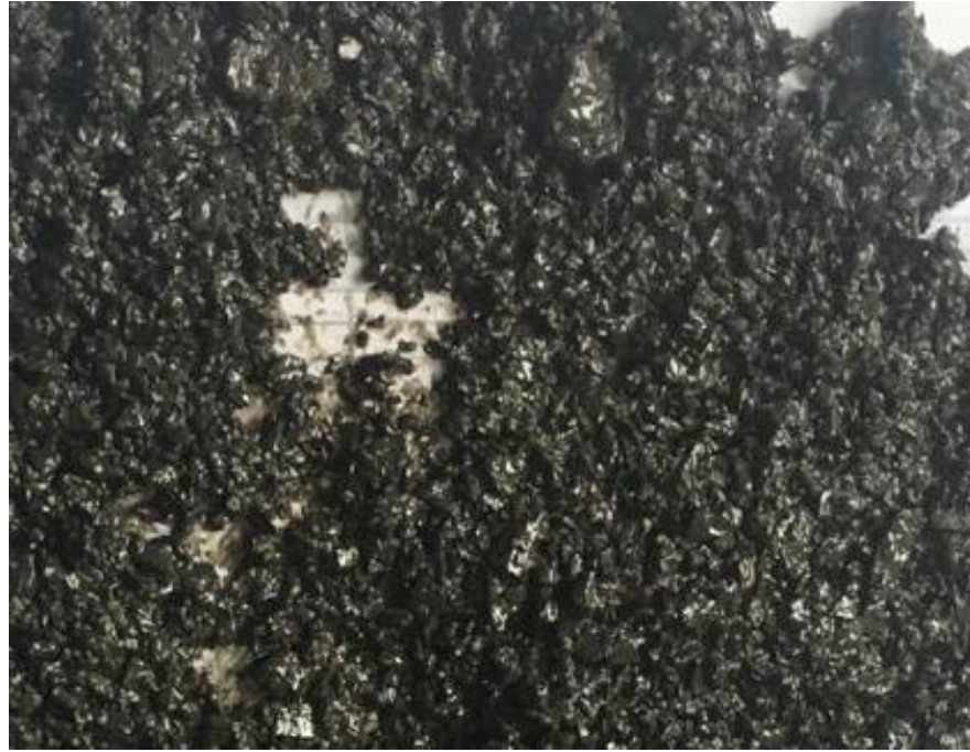
Figure 8 Case History #1 Cuttings at 95 pcf after addition of sub-micron deformable polymer
