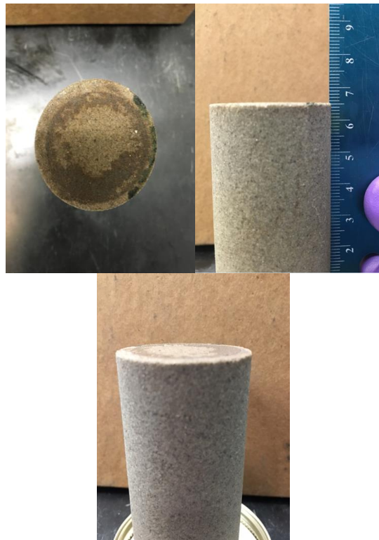
Figure 2 – Results of return permeability tests performed with core samples from the field
