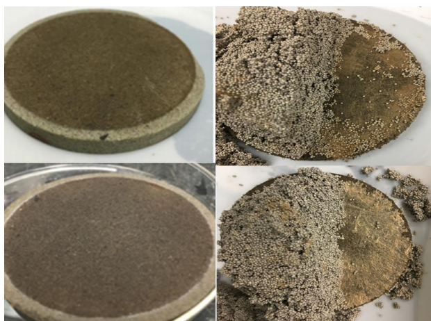
Figure 1 – Results of the breaker system action of carbonates dissolution and starches breakdown using aloxite disks: without gravel pack (left) and with gravel pack (right) demonstrating almost complete filtercake removal
