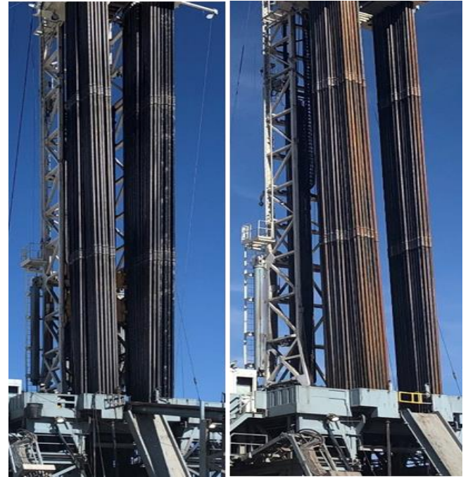
Figure 5 – Effect of Protectant (Left side: Pipes coated with protectant and Right side: Pipes not coated with protectant)
