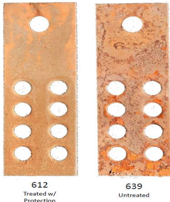
Figure 4 – Protectant-Treated Coupon on the Left and Untreated Coupon on the Right
