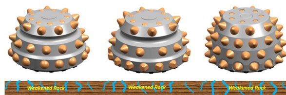
Figure 5: Comparative view of the roller cone insert layouts used in 2014 and 2017
