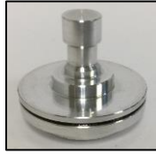
Figure 12. The cured sealant between the parallel plates.
