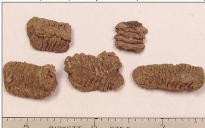
Figure 4– Gumbo shale cuttings drilled with a PDC bit, specifically in the West Delta and Viosca Knoll in the Gulf of Mexico, a reactive shale based on the mineralogy of the formation in the table above.
