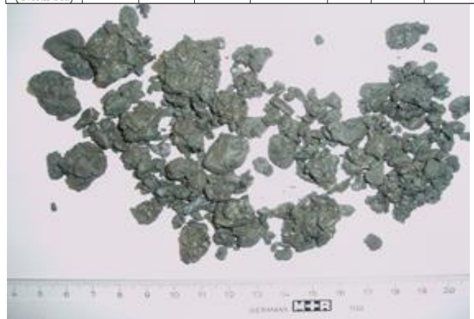
Figure 5 – Image of North Sea, green clay cuttings. Green clay is an arbitrary synonym used for reactive shale in the North Sea, the most prominent area of this clay is located in in Denmark, named Lillebaelt. Further information on the lithology of this clay can be accessed at Heilmann-Oausen et al., 1985.
