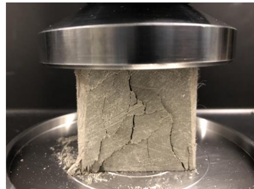
Figure 6: Result of a uniaxial compressive strength (UCS) test
