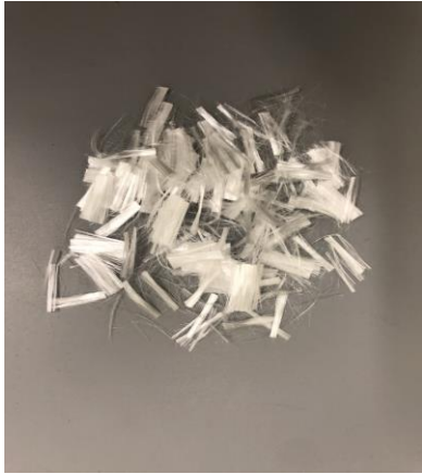
Figure 3: As received polypropylene (PP) fibers
