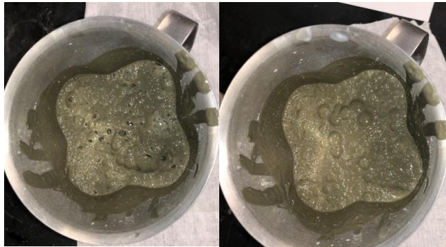
Figure 4: (Left) 9.96ppg cement without defoamer. (right) 10.61ppg cement after 1 gpt of defoamer.
