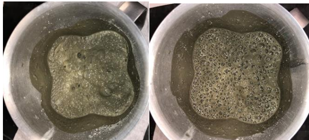
Figure 5: (Left) 9.96ppg cement without defoamer. (right) 9.32ppg cement after 1 gpt of defoamer.
