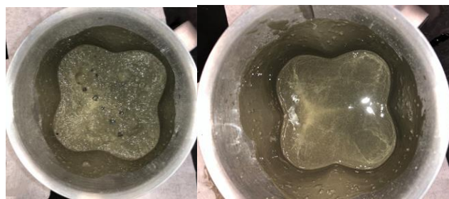
Figure 2: (Left) 9.96ppg cement without defoamer. (right) 12.00ppg cement after 1 gpt of defoamer.
