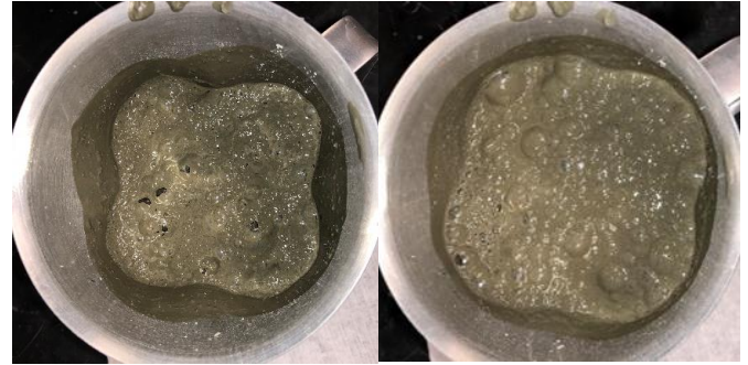
Figure 6: (Left) 9.96ppg cement without defoamer. (right) 8.52ppg cement after 1 gpt of defoamer.
