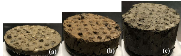
Figure 8 – Bulk hardness test: shale wafer after tests and exposed to (a) fresh water, (b) formation water, and (c) WB DIF1.
