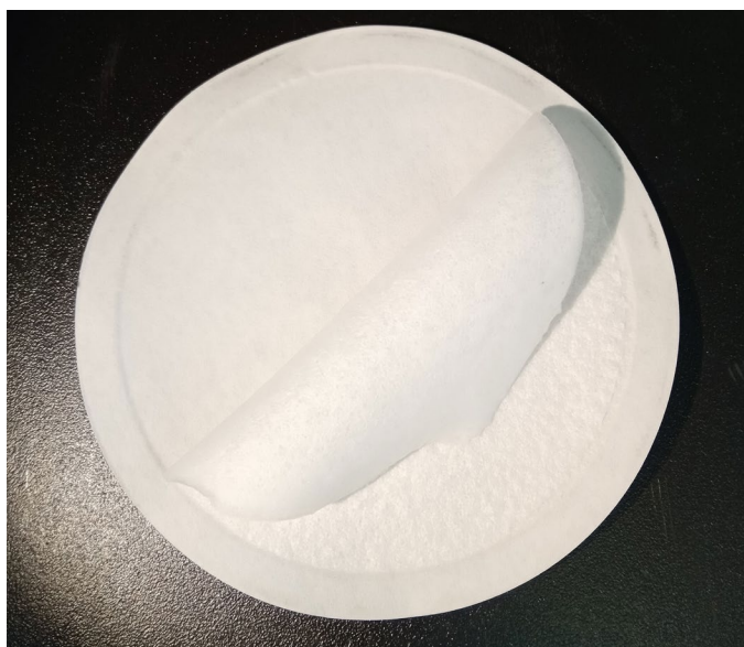
Figure 9 – Photo showing the CNF filter cake after an API filtration of a formate brine viscosified with CNF.
