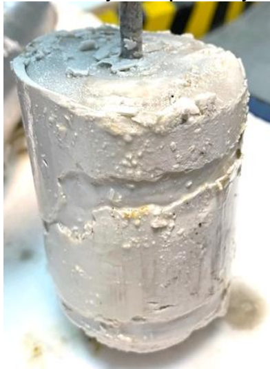
Figure C2- Image of lost circulation plug after consistometer testing. By observation, it was noticed that the plug was solid and stable (i.e., not crumble) nor was it excessively 'wet'.
