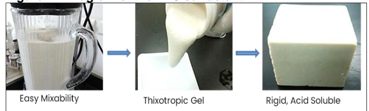
Figure 2 – Image of the ASWA in liquid form and solid form after setting.
