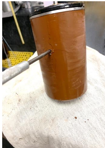
Figure B1- Images of adequately designed high density plug after 'setting' in the consistometer.
