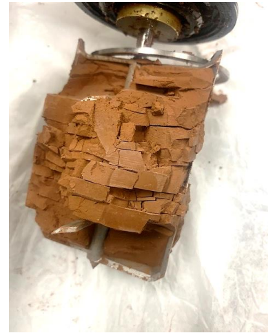
Figure B1- Images of adequately designed high density plug after 'setting' in the consistometer.
