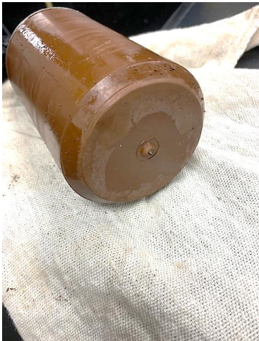
Figure B1- Images of adequately designed high density plug after 'setting' in the consistometer.
