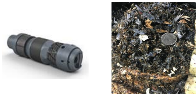
Figure 1: Composite Frac Plug and the Plug Debris after Drill Out (Bruseth and Shaffer 2020)
