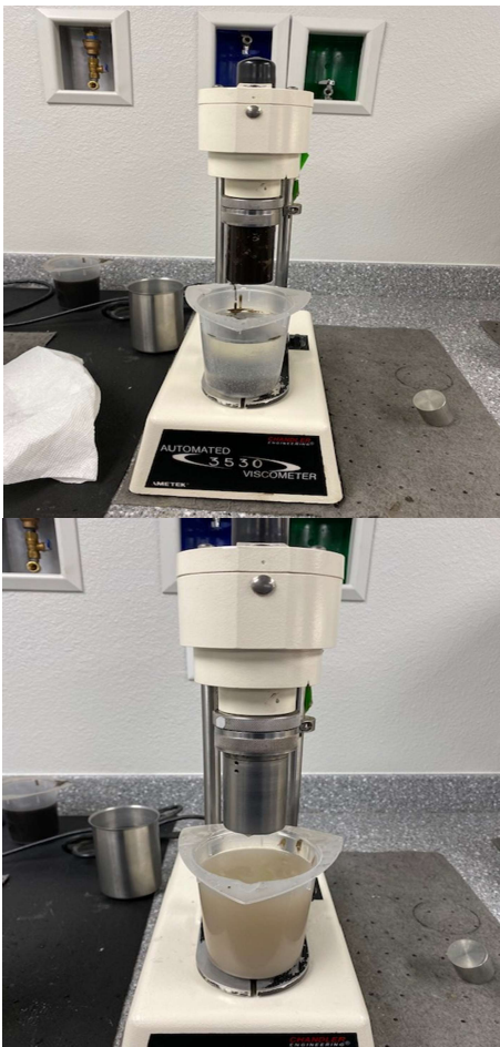
Figure 1 – Before/After Picture of Rotating Sleeve with Oil Based Mud and MCSS
