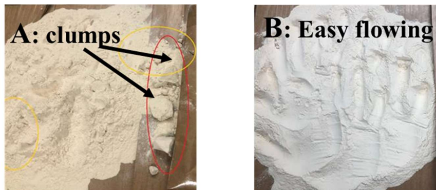
Figure 6: Flow behavior of SDA powder after opening the bags, A refers to SDA powder from 0.5 mil PE lined bag and B refers to SDA powder from 3 mil PE-lined bag
