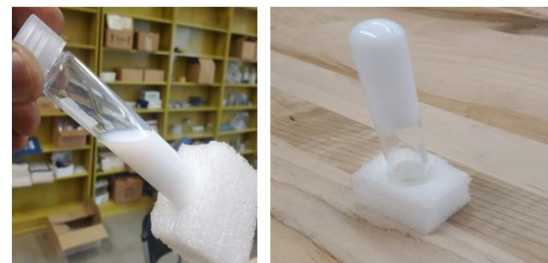
Fig 2. 15% Nano-silica gel (Before and After Gelation)
