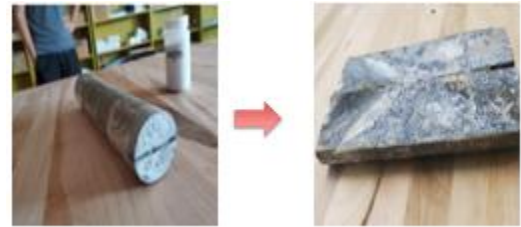
Fig 1. The Fractured Cement Core
