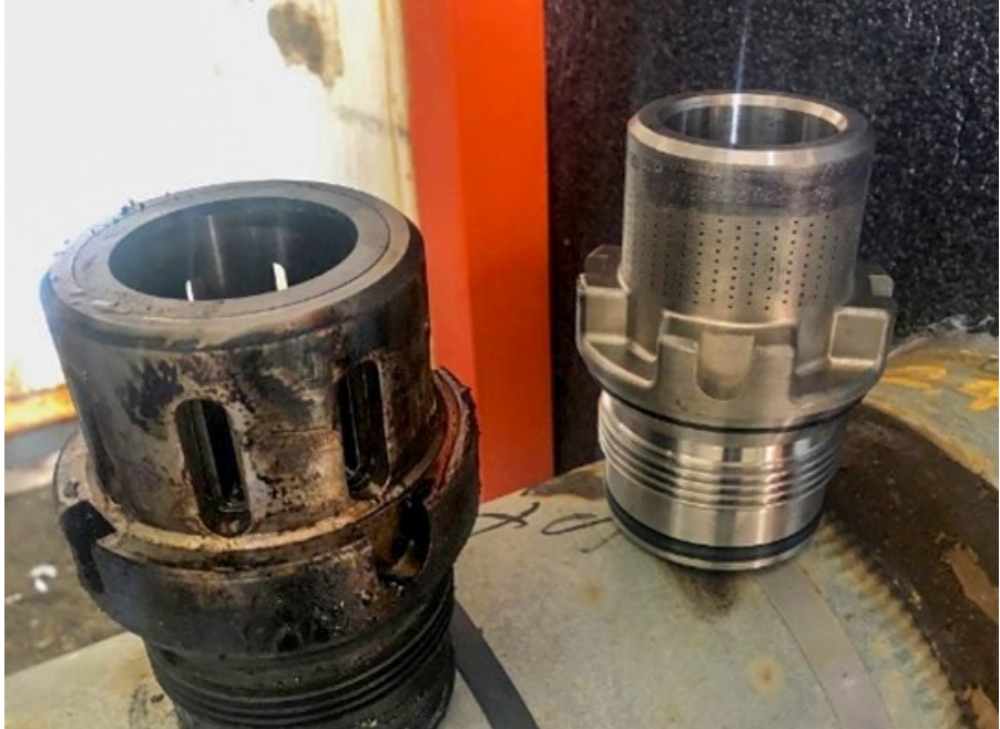
choke cage valve used as flow control devices on water injection wellheads.
