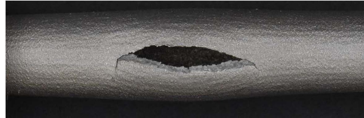
SS 316L LPBF Burst Pressure: 218 Mpa (31,673 psi)
