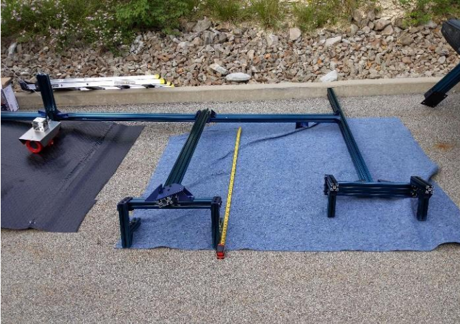
Figure 5 T-Slot Frame for Dry Shaker Mount
