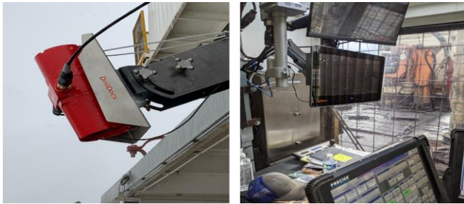
Figure 7 AI Camera on Primary Shaker and Video Touch Screen at Driller Chair
