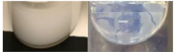
Figure 2 – Initial polymer system appearance (left) and appearance after micelle formation (right).
