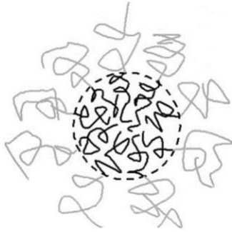
Figure 4 - Graphic representation of a micelle formed by novel polymer in base oil.
