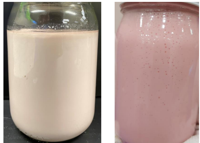
Figure 2. (left) New low-viscosity direct emulsion and (right) old xanthan-based solution.
