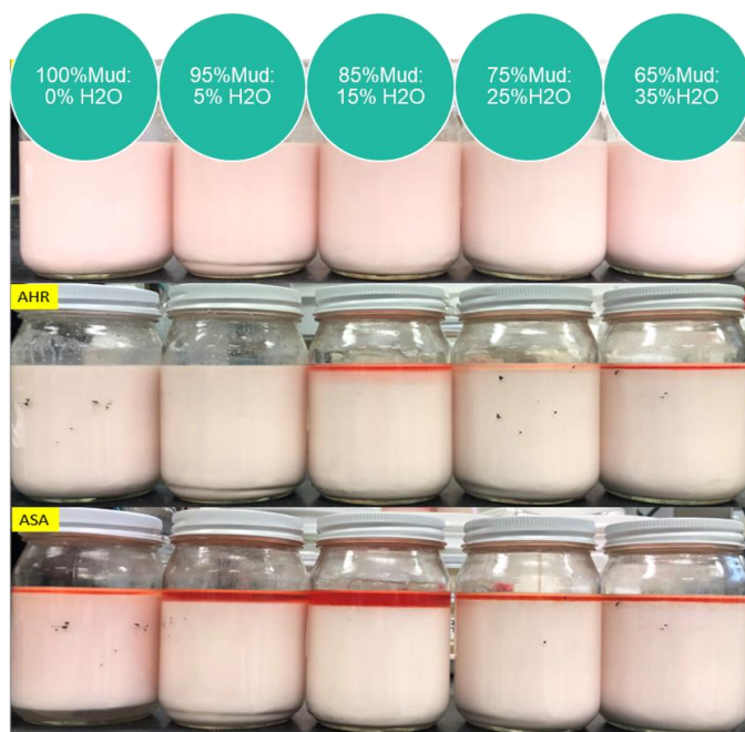
Figure 4. Surfactant-stabilized direct emulsion at various brine-diesel-ratios showing good initial, AHR, and ASA stability
