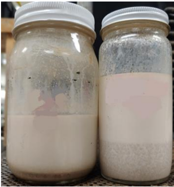
Figure 8. Solids-laden direct emulsion(left) and flocculated solids(right) with emulsion still intact.
