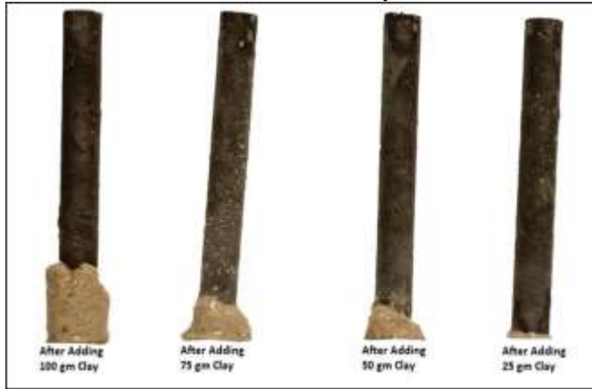
Figure 4: Clay accretion profile in WBM with KCl and without AFR
