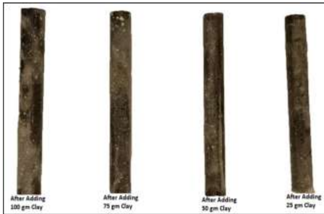
Figure 5: Clay accretion profile in WBM with KCl and AFR
