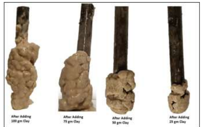
Figure 3: Clay accretion profile in WBM without both KCl and AFR
