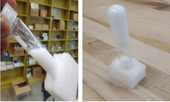
Figure 2: Appearance of Nano silica gel (a) Before Gelation (b) After Gelation
