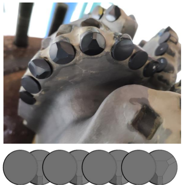
Figure 4: Illustration of some cutter layout practices tested in the Laboratory
