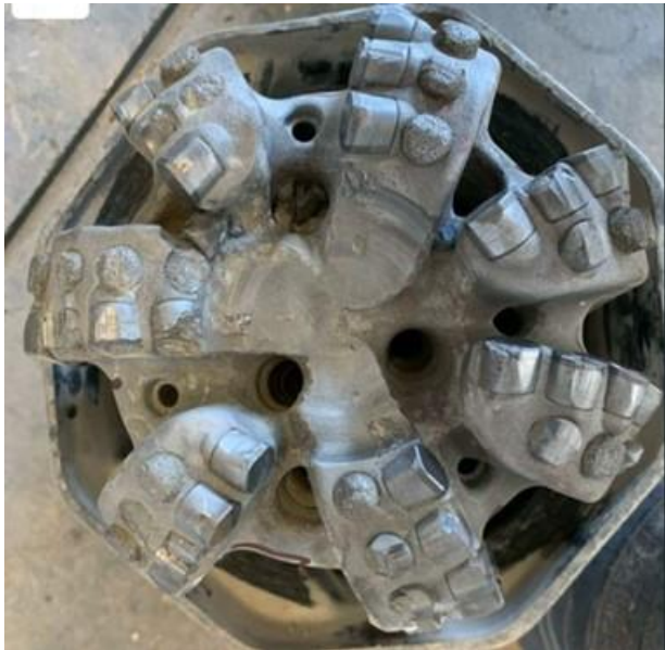
Figure 14B: Test Bit B Dull fitted with standard planar faced cutters
