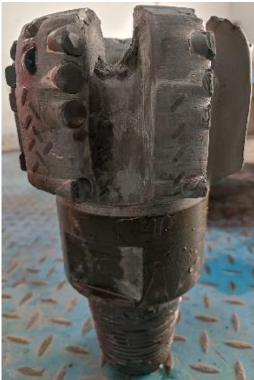
Figure 8 – Dull Photo of Bit with Multi-faceted Cutters
