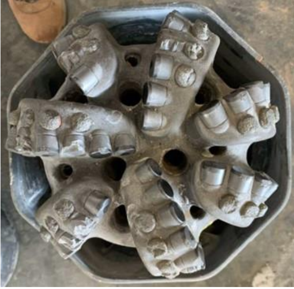
Figure 14A: Test Bit A Dull fitted with multi-faceted shaped cutters
