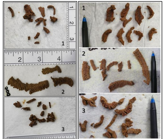
Figure 5 – Cuttings from intact rock (left) and pre-grooved rock (right).
