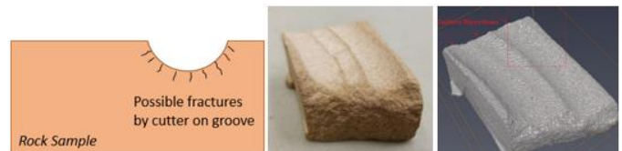
Figure 10 – Illustration of the possible existence of fractures left on the grooves that may reduce the cutting forces for the next round of cutting; studied by the author in 2019.
