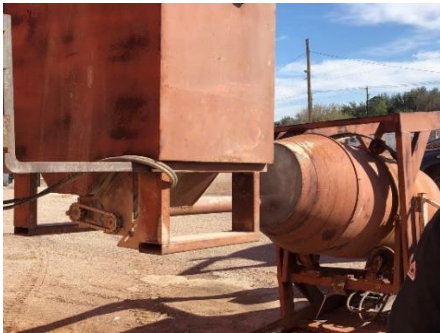
Fig. 4: dry components being mixed into activating solution
