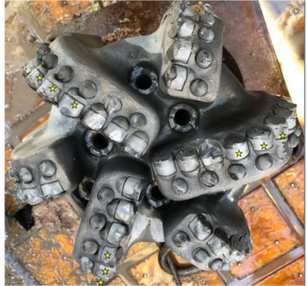
Figure 11 Dull condition of 2nd corrosion resistant cutter test
