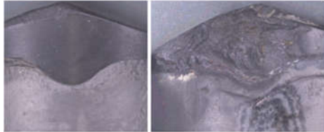
Typical corrosion damages on two baseline cutters from the same bit
