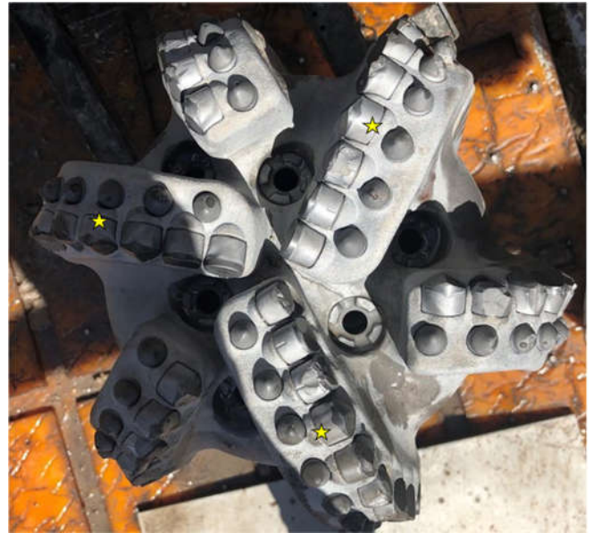
Figure 7 Condition of Dull after run. Yellow stars designated corrosion resistant cutters
