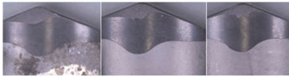
Side views of three cutters on modified substrate, showing negligible corrosion damages
