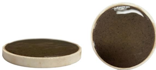
Figure 12 – Filter cake generated with 6 lb/bbl of Blend #4 on a 3-micron aloxite disk, resulting in 9 cc/30min filtrate
