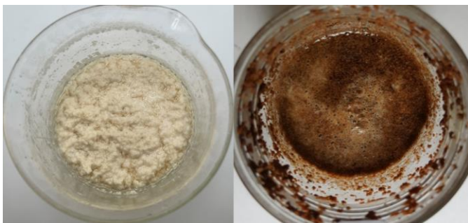
Figure 6 – Incompatibility examples of experimental lubricants cheesing (left) and greasing (right)
