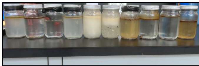
Figure 7 – Jar testing of various lubricants after hot rolling at 150°F
