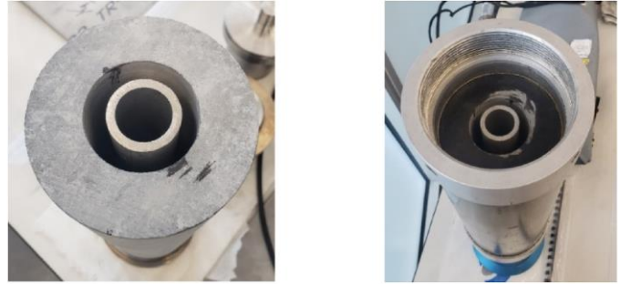
Figure 6 Wellbore Model for cement placement
