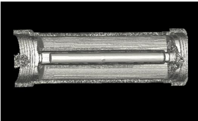
Figure 9 3D Volume image of the wellbore model.
