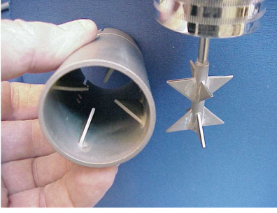
Figure 1. Photo of actual viscometer with intermeshing teeth that was adapted to a conventional bob and sleeve viscometer.
