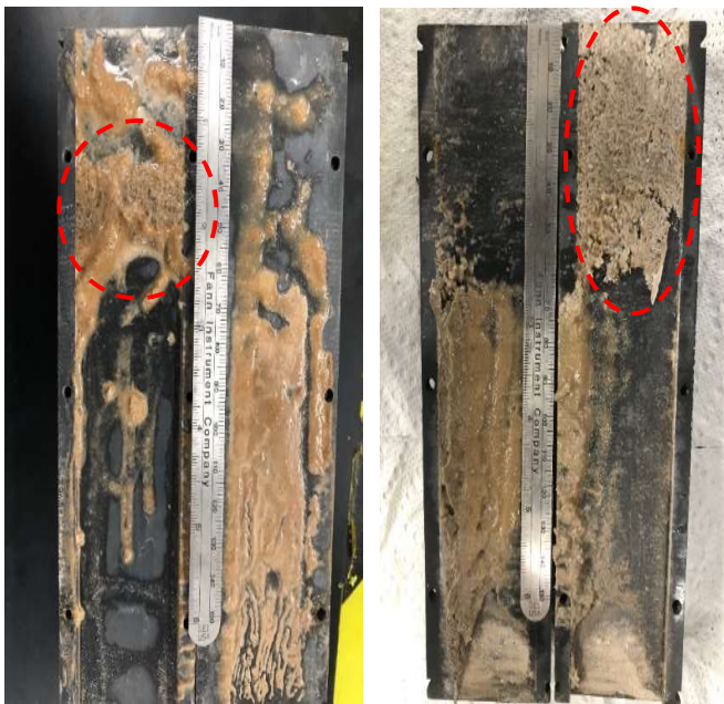
Figure 9 a) sealing effect before shape recovery; b) sealing effect after shape recovery.
