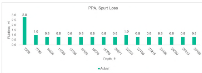
Figure 13 (a) – Spurt loss from PPA test at different depths for Well # B at different depths during the drilling
