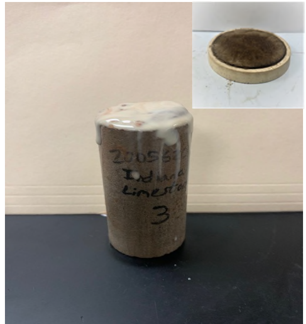
Figure 6 (a)- Limestone Core with filter cake for the Mud without NP
