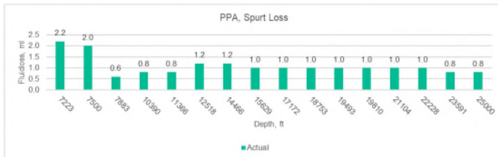
Figure 12 (a) – Spurt loss from PPA test at different depths for Well # A at different depths during the drilling
