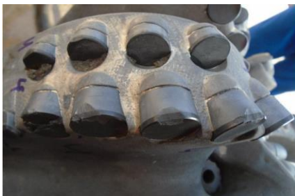
Figure 2. Damaged bit structure previous runs
