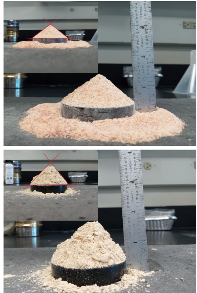
Figure 4 – Angle of repose test images for SSA (top) and SAn1 (bottom)
