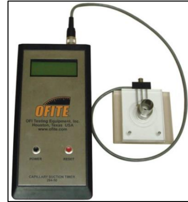
Figure 5: Capillary suction timer. Photo: Courtesy of https://www.ofite.com/products/wastewater/meters-52/capillary-suction-timer .
