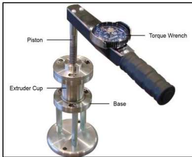
Figure 3: OFITE bulk hardness tester. Photo: Courtesy of https://www.ofite.com/products/drilling-fluids/swelling/bulk-hardness-tester .
