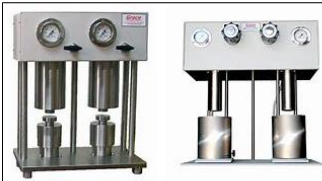
Figure 4: Grace M4600 LSM and Pelletizer. Photo: Courtesy of https://www.gic.com/M4600.php .
