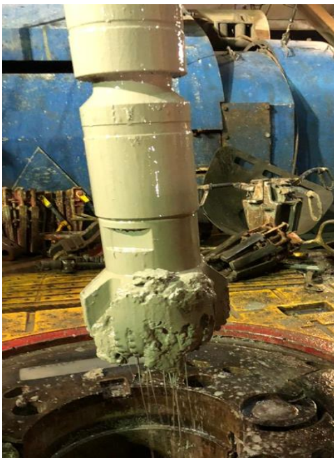
Figure 6 - BHA after pull out of the hole
