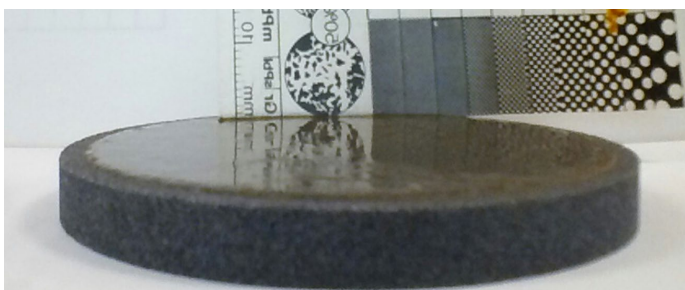
Figure 5 – Photo of the filter cake from the Martin Linge field mud after an HP/HT fluid loss test on a 50-µm disk at 135°C (275°F).
