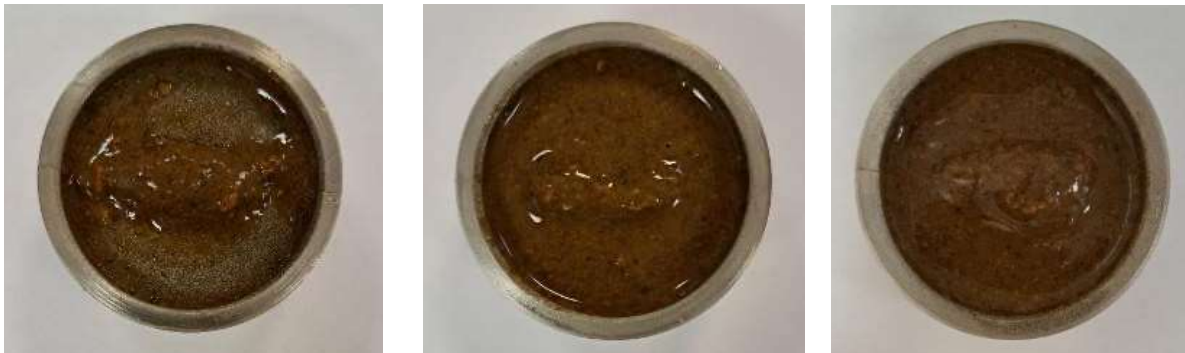
Figure 4 – 8.7-lb/gal spacer with LCM. Left to right: 1-mm, 2-mm, and 3-mm slot apertures.
