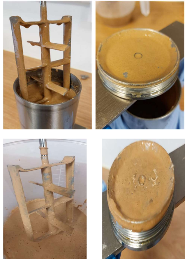
Figure 8 – Visual observation after dynamic testing. Unweighted, 8.7 lb/gal (top) and 11.5 lb/gal (bottom) slurries.
