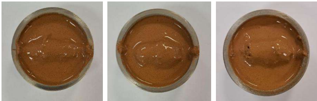
Figure 5 – 11.5-lb/gal Spacer with LCM. Left to right: 1-mm, 2-mm, 3-mm slot apertures.
