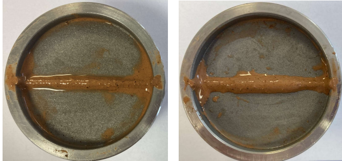
Figure 3 – 11.5-lb/gal spacer tested on 200- \mu\text{m} slot disk (left) and 350- \mu\text{m} slot disk (right).
