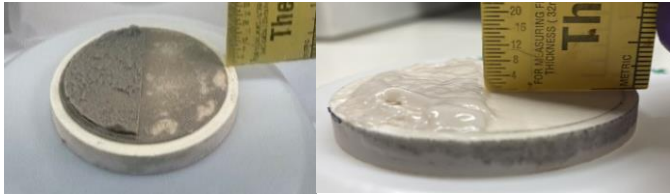
Figure 3. A comparison of the 1- hr filtercakes of new DIF (left) versus used DIF (right).
