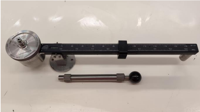
Figure 1. Increased-accuracy pressurized mud balance
