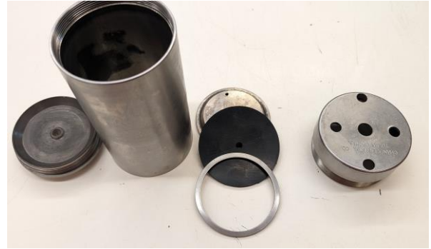
Figure 13. Consistometer cell without paddle or shaft, used for HTHP sag measurement
