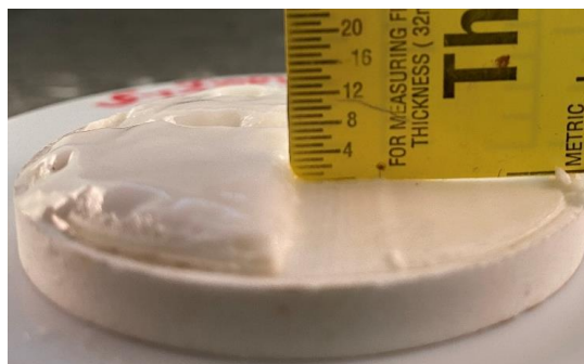
Figure 12. The 16 hr filtercake of the WB-DIF at 8,000 psi, 360 °F.
