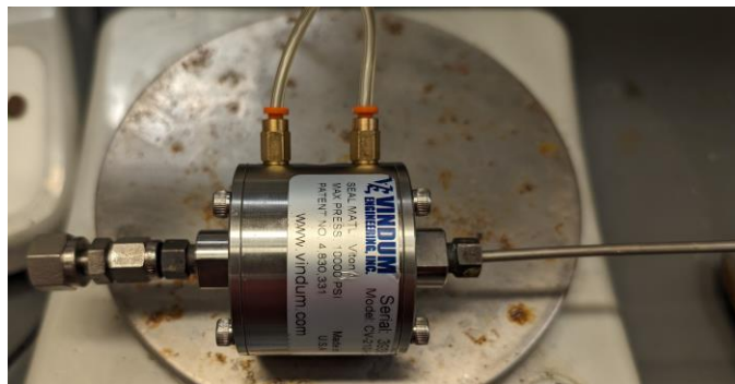
Figure 8. Air-operated constant flow valve
