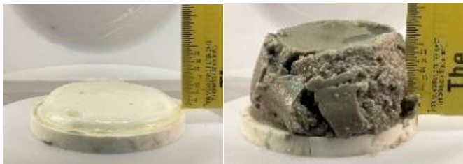
Figure 4. A comparison of the 16- hr filtercakes of new DIF (left) versus used DIF (right).
