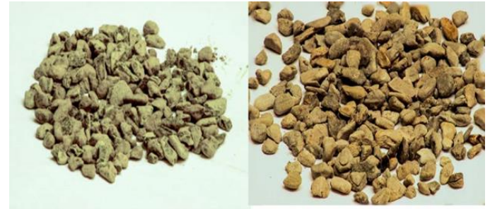
Figure 8: Cuttings on shakers-from section 12 1/4"
