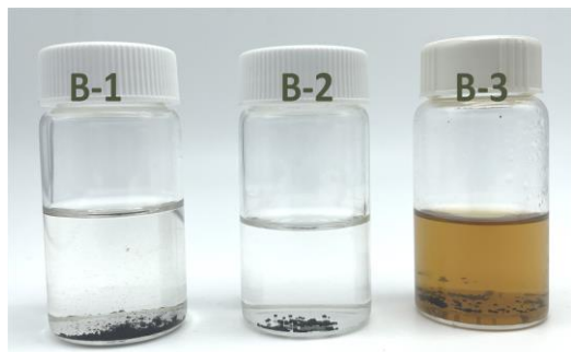
Figure 4: Effect of biosurfactant on asphaltene dissolution (Vial B1: asphaltene + heptane, B2: B1 + ethanol, and B3: B2 + biosurfactant)
