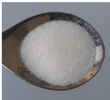
Figure 3: Styrene plastic spherical beads lubricant
