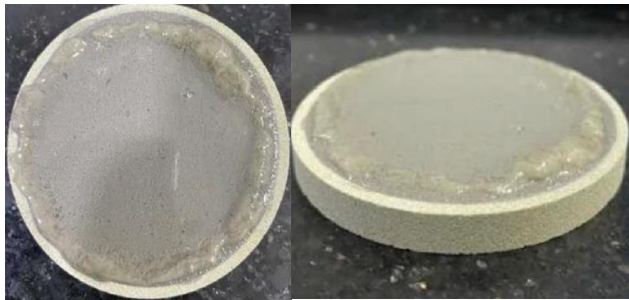
Figure 6: Filter cake generated on 20 µm ceramic disk after PPT
