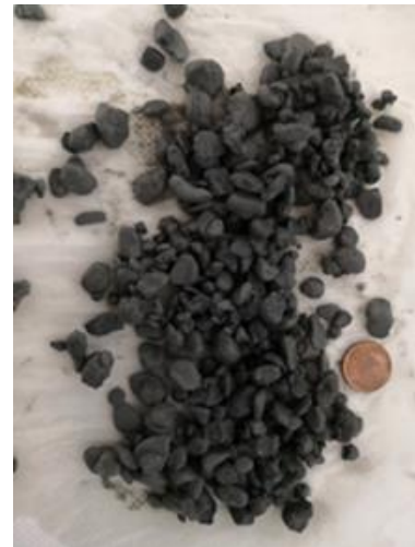
Figure 13: Cavings observed on shakers
