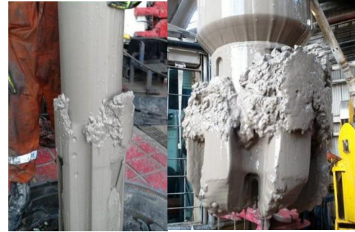
Figure 15: Bit and BHA on surface with clear indication of Bit Balling
