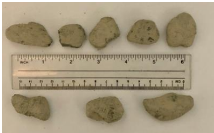
Figure 14: Cavings seen on shakers while circulating at 13 3/8" CSG shoe
