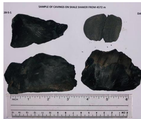
Figure 17: Cavings on shakers while circulating at 4572 m while POOH
