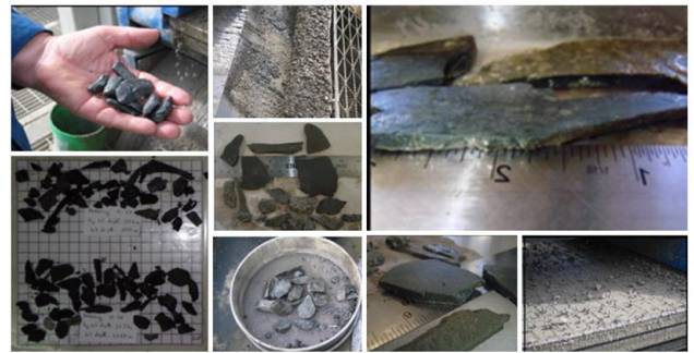
Figure 6: Cavings from Well#5 (Angular, Splintery & Tabular)
