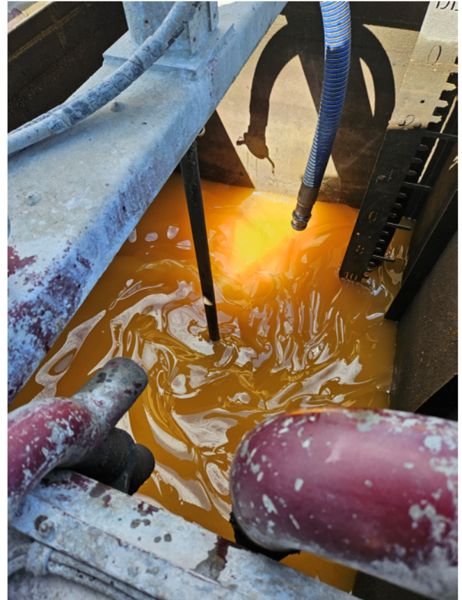
Figure 8 - Resin Mixing on Cementing Pump Truck
