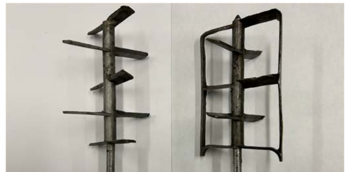
Figure 3 – Modified Paddle vs. API Paddle for Thickening Times
