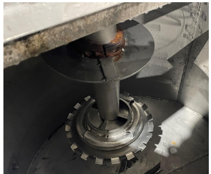
Figure 6. High shear LSL tank interior and mixer blade
