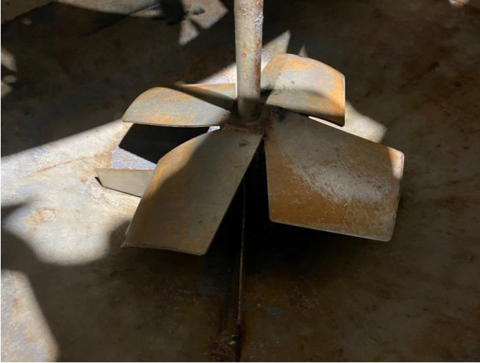
Figure 7. Low shear tank interior and paddle mixing blade.
