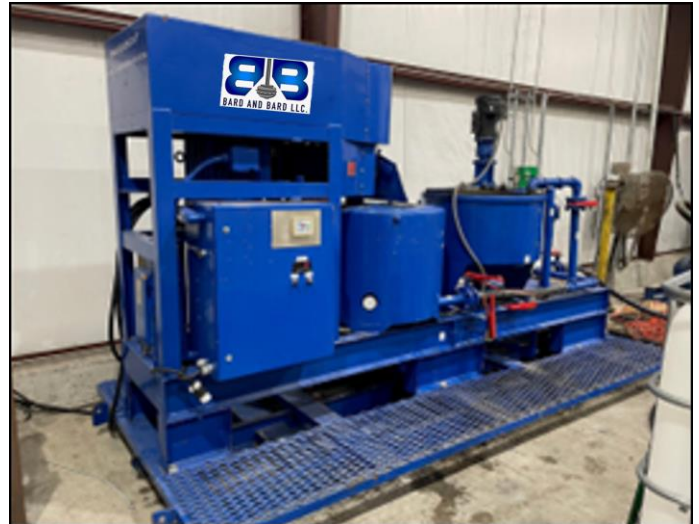
Figure 5. Commercial pilot mixer equipped with high shear LSL mixer and low shear mixer.
