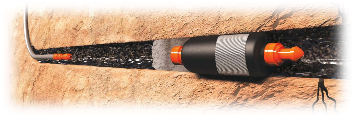
Figure 2 – Depiction of an Inflatable Open Hole Bridge Plug deployed in horizontal open hole
