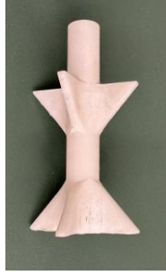
Figure 3. 3D printed FYSA with ceramic materials.
