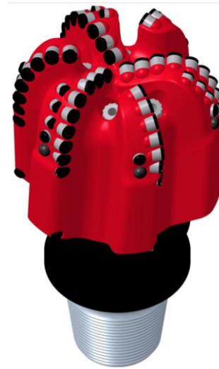
Fig 7: Test bit of 8.75" in size that was used for the field validation
