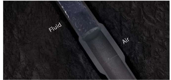
Figure 3 – Fluid and air sections in the flotation collar.
