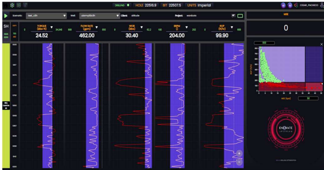
Figure 1- Maintaining parameters within the optimal range, as shown here, ensures a high Rate of Penetration (ROP), leading to faster and more efficient drilling operations.
